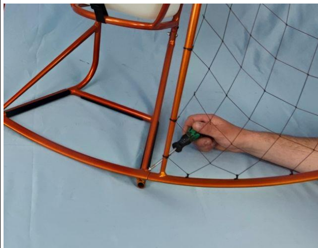
and gently lock them with the screwdriver (size PH1) and torque as indicated on the torque table (size: M4)
