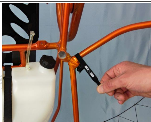
The velcro that runs around the tube prevented the screw from unscrewing with the vibrations
